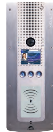
XE PAD VIDEO MI EVO Audio video Full IP/SIP entry station with names scrolling and upgradeable Mifare+ and Bluetooth reader DDA compliant REF 590.3600
