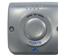
BP SORTIE H ZAMAK Zamak exit push button - DDA compliant (IP54 - IK09) REF 330.1200 > Sound information through a buzzer and a green led for door opening information > Permanent blue led lighting > Integration inside housing box Ø 60 mm > Optional base for surface mounting (REF 330.1250) > Dimensions 90 x 90 x 24 mm (96 x 95 x 39 mm with base) > Power supply 12/24V not included
