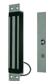
VENTOUSE ENCASTRE 300KG 24V Magnetic lock flush mounting standard compliant NFS61937 REF 320.1200 > Holding power 3000N > Length 230 mm > Width 38mm > Depth 27mm > 24V
