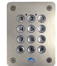
CLAVIER AUTONOME BRAILLE Standalone coded keyboard with backlit (blue) keys with Braille diameter 16 mm - 2 relays REF 330.0200 > Led and operating buzzer > Stainless steel vandal proof front panel > Flush mounted > Programming through the front panel via a master code > Dimensions 135 x 100 x 2.5 mm (flush-mounted with flush box D 40 mm) > 140 x 105 x 60 mm (surface-mounted with optional surface box - REF 330.0150 -) > Power supply 12V not included
